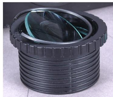
Flip the focus lens barrel over and insert the lens. Carefully insert the retainer ring. Please do this very carefully. Make sure retainer ring is in correctly, flesh against the lens. Now you can screw the focus lens back into the H2O IR.
